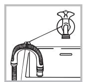
The drain hose may be connected to an under-sink trap. Before connecting the drain hose from the machine ensure that any blanks or removable ends have been taken off the spigot.
